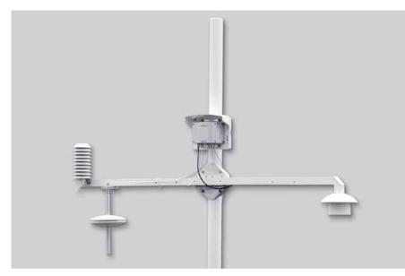
The HMT337 and PTU307 feature warmed probe technology. Installed with the HMT330MIK kit either one forms the right choice for reliable humidity measurement in humid weather conditions.
