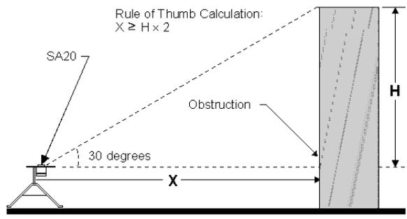
**Figure 27 SA20M Vertical Obstruction (Side View)**
