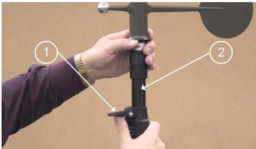
**Figure 37** Extending the Telescopic Mast
