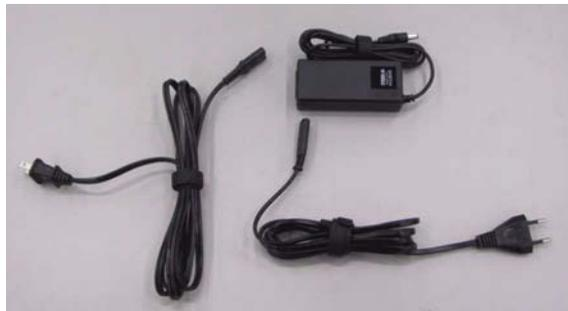
**Figure 9** Mains Power Supply Module QMP211
