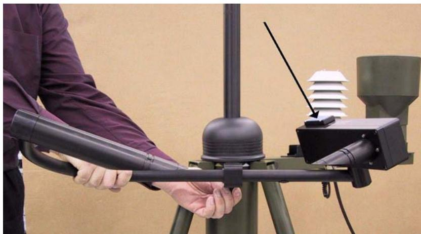
**Figure 55** Installing PWD22M (Arrow Pointing to Rain Detector Plate)
