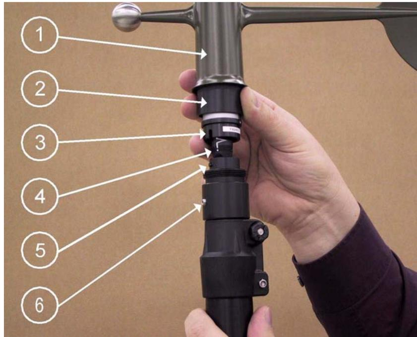
**Figure 35 Wind Sensor Attachment**
