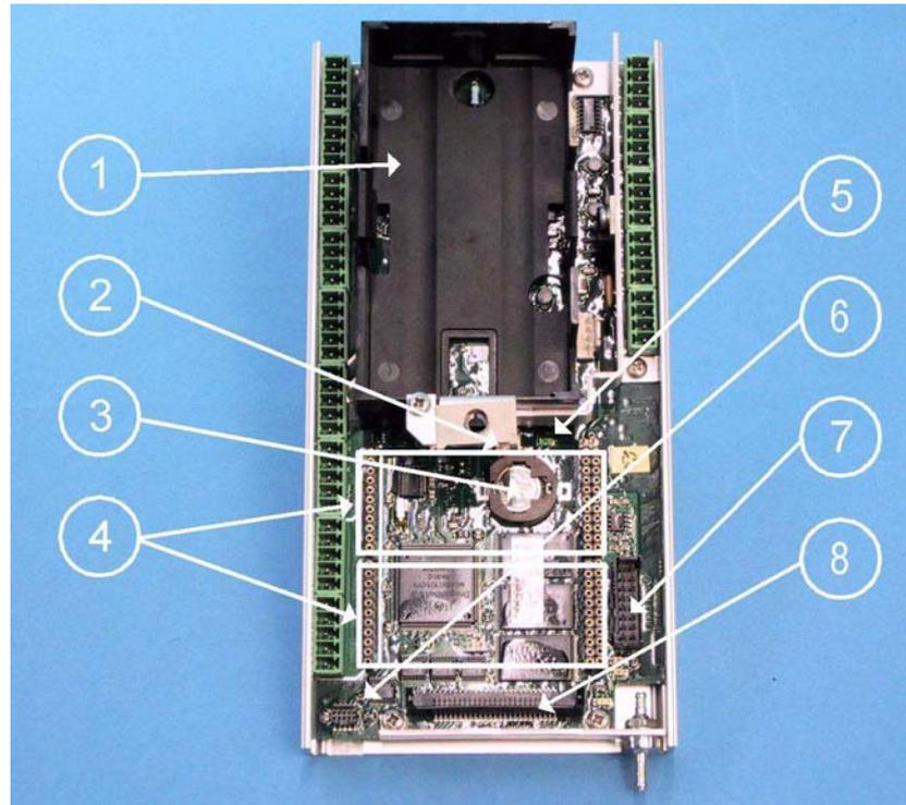
**Figure 6** AWS Logger QML201 without Cover
