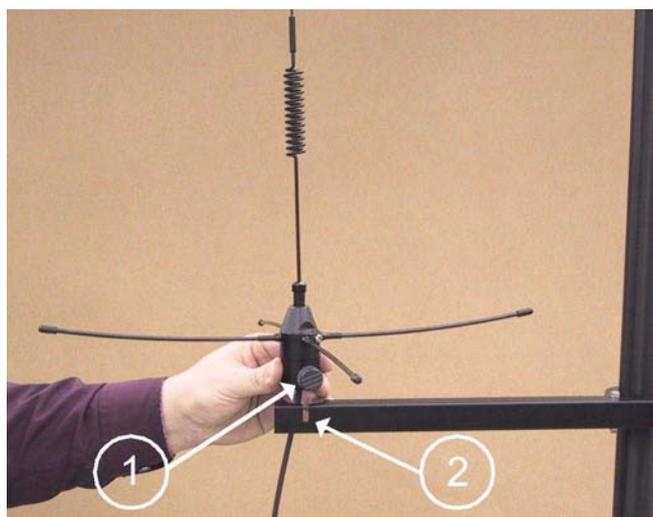
**Figure 41** Installing UHF Antenna to Arm
