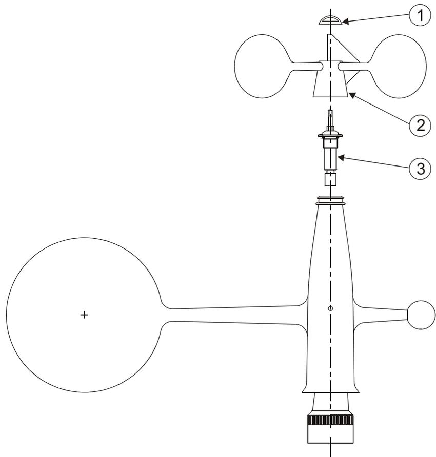
**Figure 90** WMS302M Sensor Assembly
