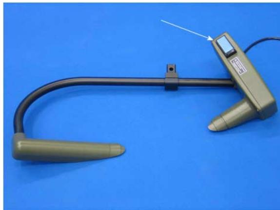
**Figure 89** Present Weather Detector (Arrow Pointing to DRD)
