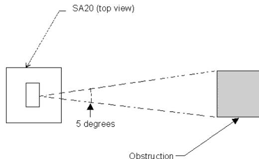
**Figure 28 SA20M Horizontal Obstruction (Top View)**
