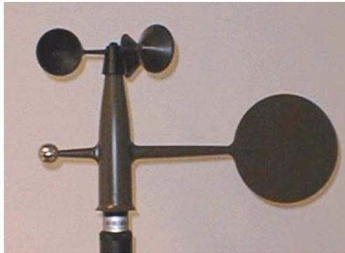
**Figure 15 Combined Wind Speed and Direction Sensor
