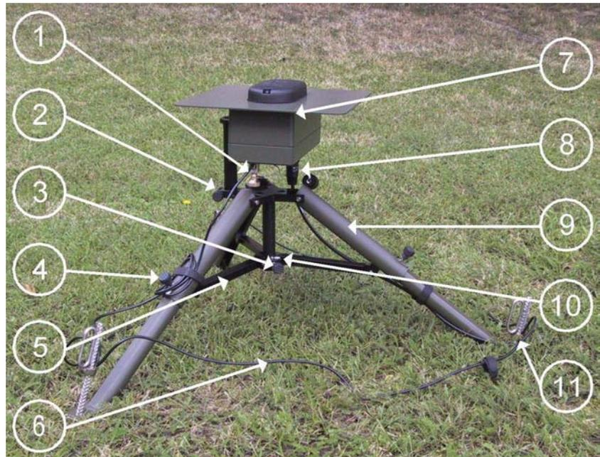
**Figure 59** Lightning Detector SA20M with Grounding Net
