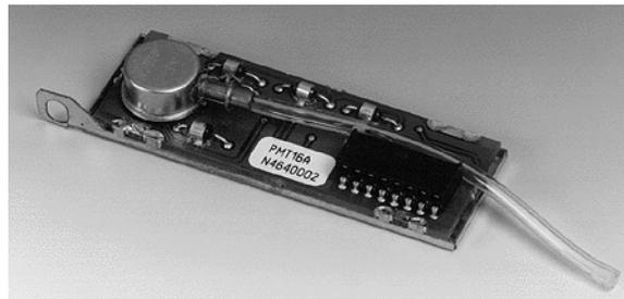
**Figure 18**      **Pressure Sensor PMT16A**
