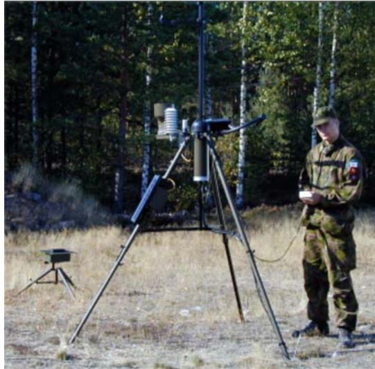
**Figure 2 Complete TACMET MAWS Can Be Installed and Operated by One Person**
