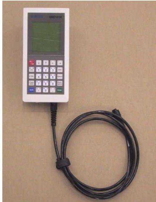
**Figure 11 Handheld Terminal QMD101M**
