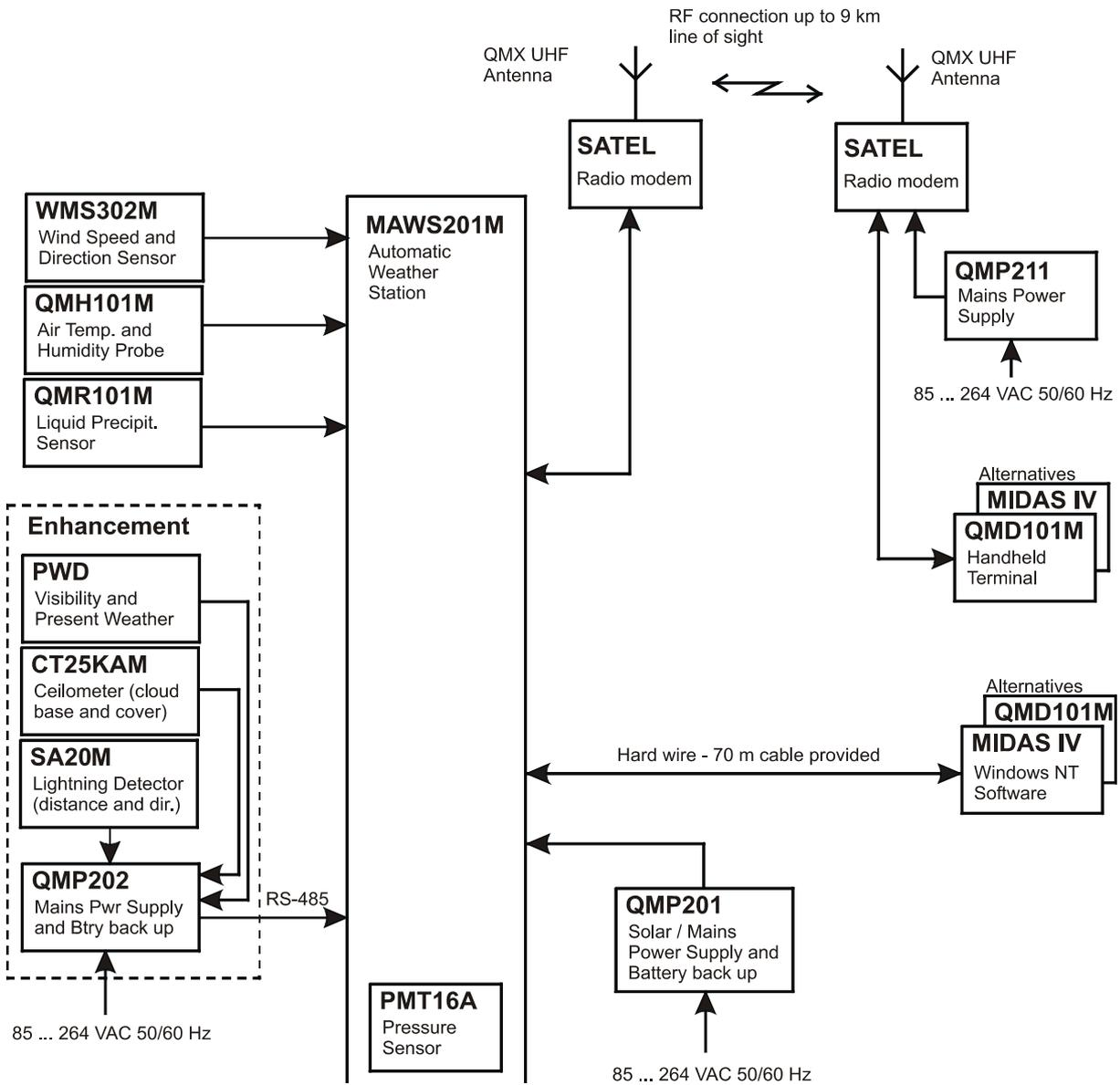
**Figure 1 Block Diagram of the Basic System and Enhancement**
