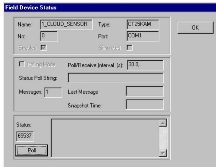
**Figure 86** Sensor Details in Field Device Status Window
