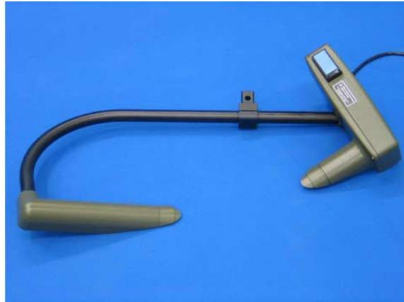
**Figure 19 Present Weather Detector PWD22M**
