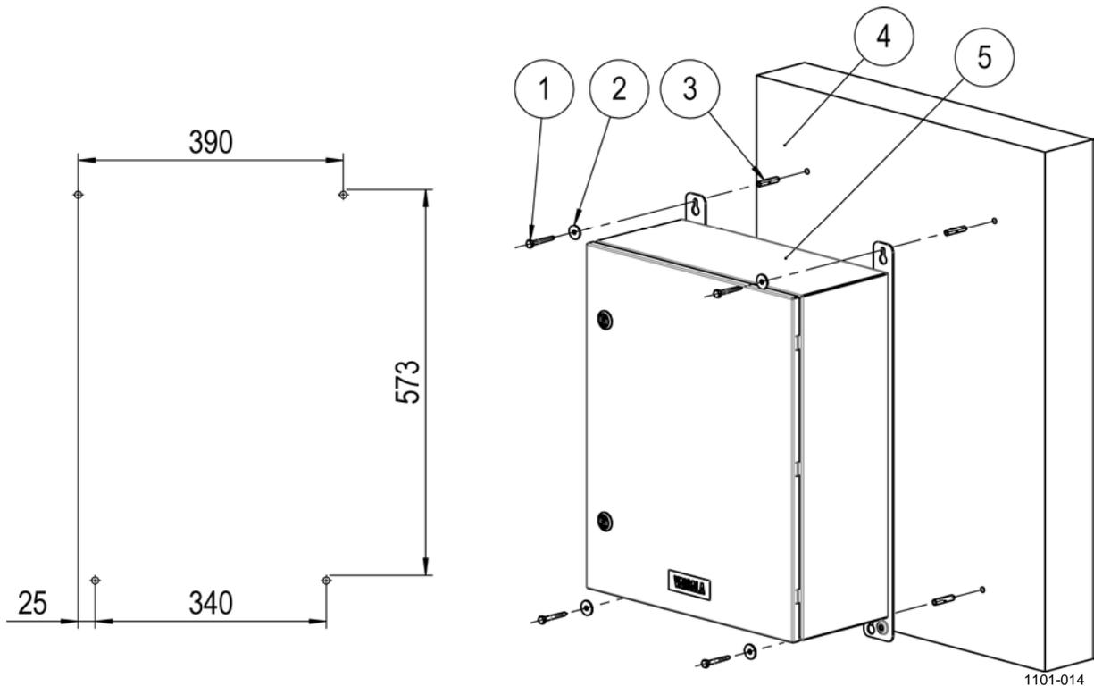
**Figure 49** Installing Enclosure to Wall
