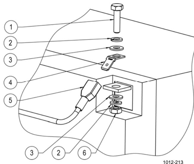
**Figure 55** Connecting Battery
