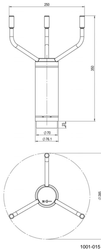
**Figure 134 Ultrasonic Wind Sensor WMT703 Dimensions in Millimeters**
