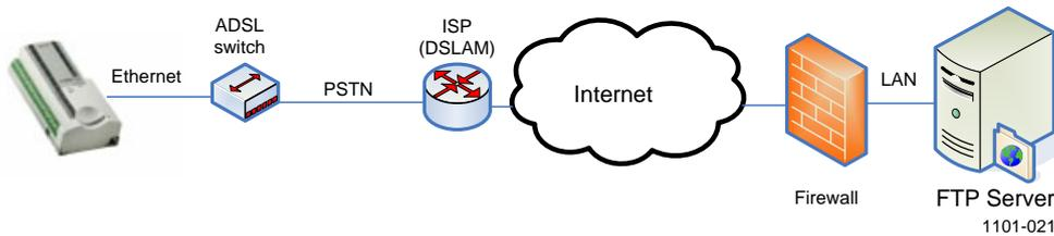
**Figure 73 Example FTP Transmission**
