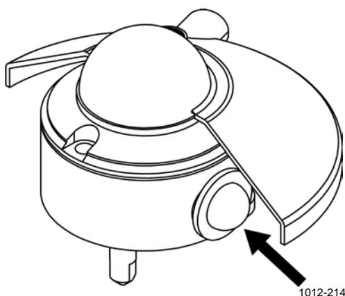
**Figure 109** Pyranometer CMP6, Arrow Points to Drying Cartridge
