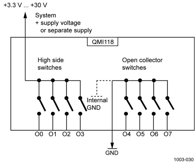
**Figure 131 Digital I/O Module Wiring Diagram (Digital Outputs)**
