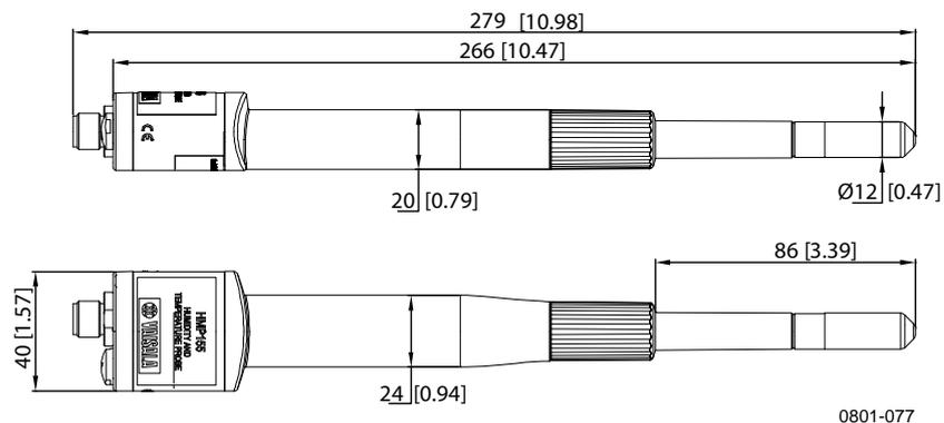
**Figure 136 Probe Dimensions**
