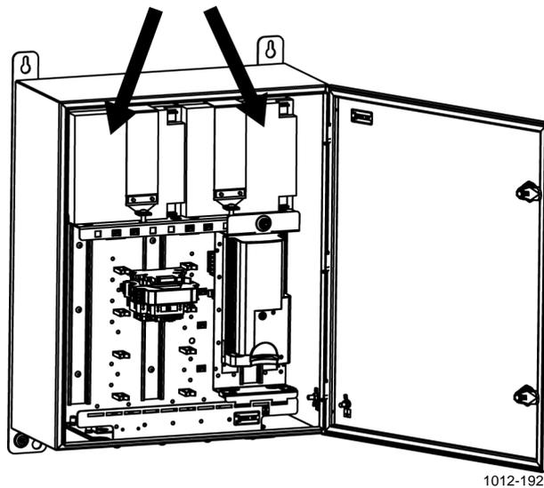
**Figure 50 Backup Batteries Positioned Correctly**
