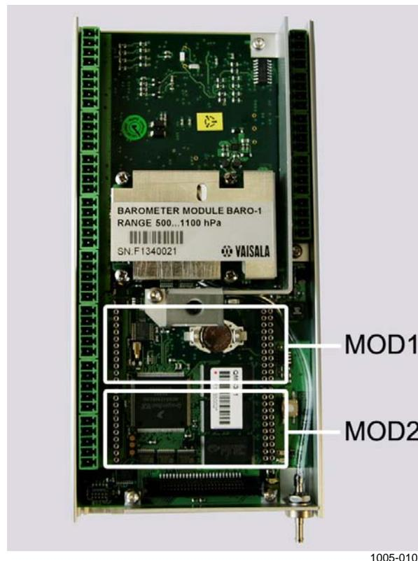
**Figure 113** Communication Module Placement
