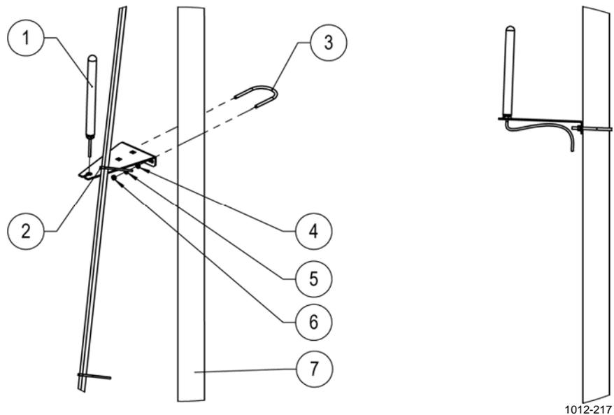
**Figure 33 GSM/GPRS Antenna Installation**
