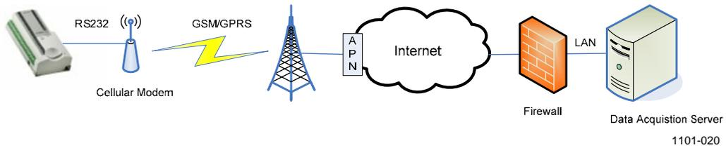
**Figure 71** Example TCP-Socket for Message Transmission
