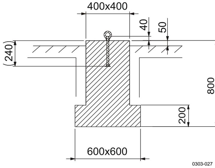
**Figure 7 Concrete Block for Guy Wire (Dimensions in mm)**
