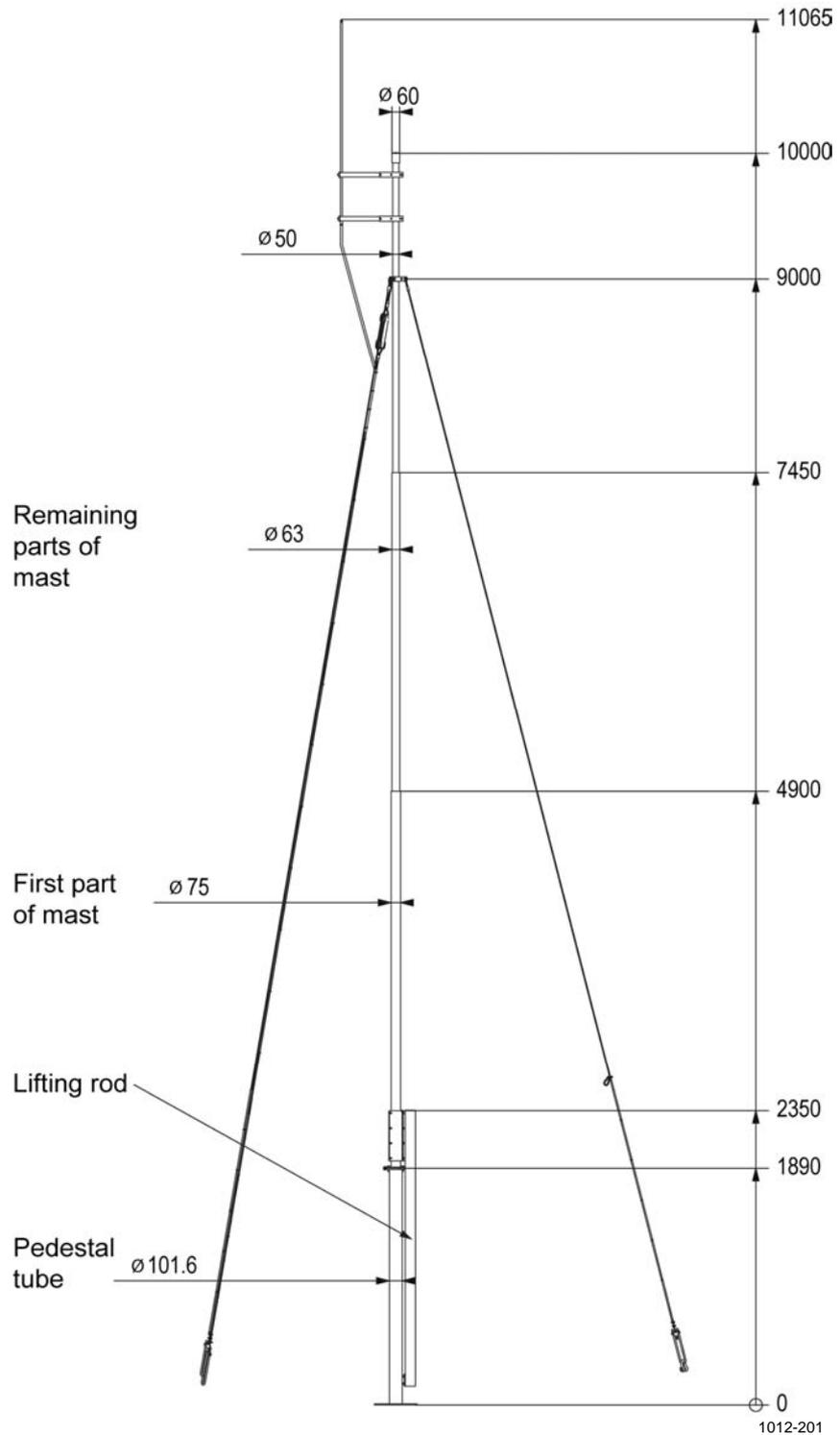
**Figure 12 DKP210 Mast Dimensions (in mm)**
