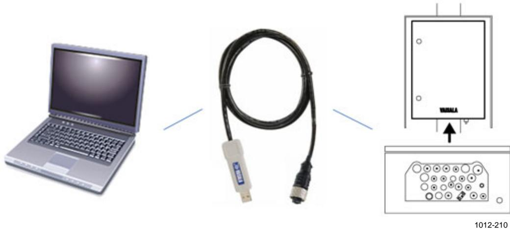
**Figure 57** Connecting Maintenance Cable
