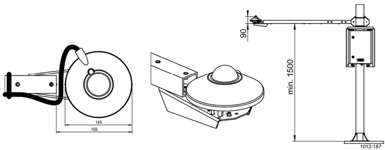
**Figure 42** Pyranometer CMP6 Dimensions, Pyranometer CMP6 Installed
